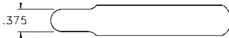
Figure 1 - NARROW THE REQUIRED FEELER GAUGE AS SHOWN. LEAVE A SMOOTH ROUND EDGE.
